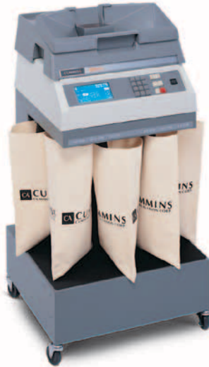
The JetSort® 4601 floor model in use at the Fairlawn facility counts up to 4,500 coins per minute.
